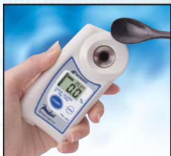
①Place the sample onto the prism surface.
