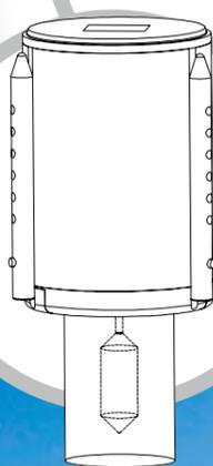
Placing the instrument directly on the included beaker
