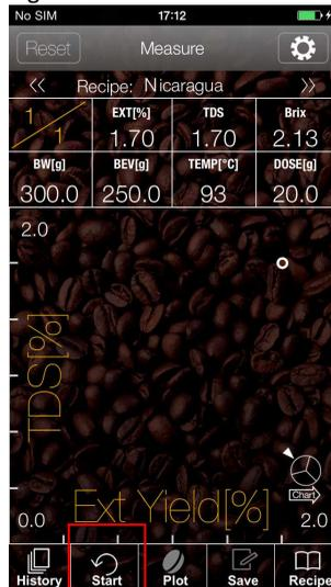
**memo** Up to 10 entries can be temporarily saved. Once the number of entries is exceeded, data will be erased, starting with the oldest data entry. You can keep track of the entries using the counter at the top-left corner and confirm the number of entries by tapping the “<< >>” to select through temporarily stored data.
