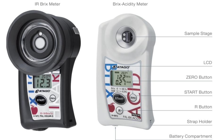
A combo set that includes PAL-HIKARI, a non-destructive IR Brix Meter that can measure the sugar content just by being pressed against the fruit, and PAL-BX|ACID, a Brix-acidity meter that can measure the sugar content of squeezed fruit juice is now available. Special scales are available for each fruit. Choose the appropriate combo set.
