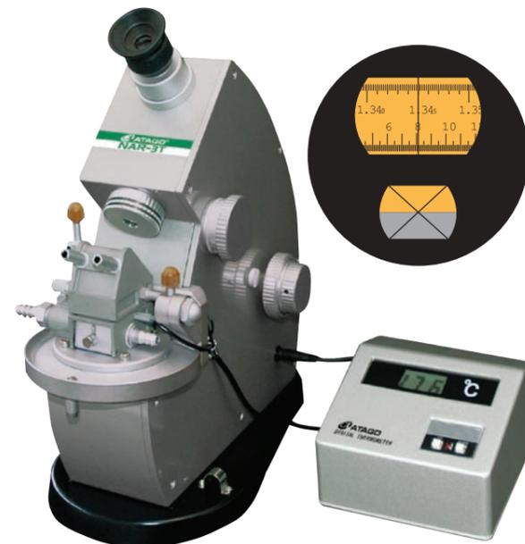
The NAR-3T is the unit with the highest degree of precision and accuracy among the Abbe Refractometers. It was developed to give improved measurement accuracy and ease of use. This was achieved by making fundamental improvements to the optical system and utilizing a larger scale, which allows for a refractive index scale measurements of up to 0.00005. Incorporating a high intensity lamp and using a double control knob gives quick and more accurate control.
