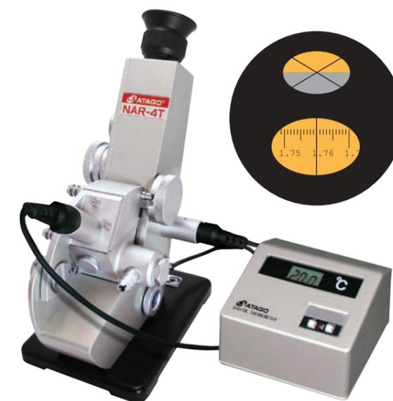
Research and Development on new materials for modern technologies is being actively conducted in every industry. Many of these materials (especially polymer film and related materials) are of high refractive index - often too high for the existing Abbe refractometers. These can now be measured with the nD 1.4700 to 1.8700 range of the NAR-4T.
