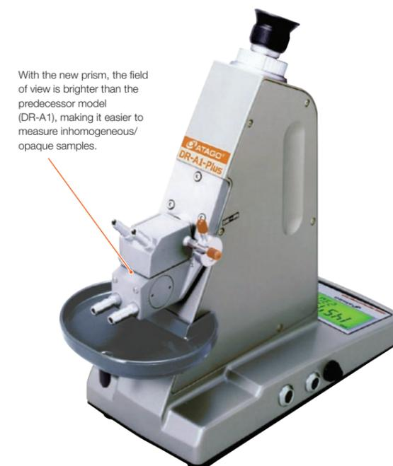
With the new prism, the field of view is brighter than the predecessor model (DR-A1), making it easier to measure inhomogeneous/ opaque samples.
