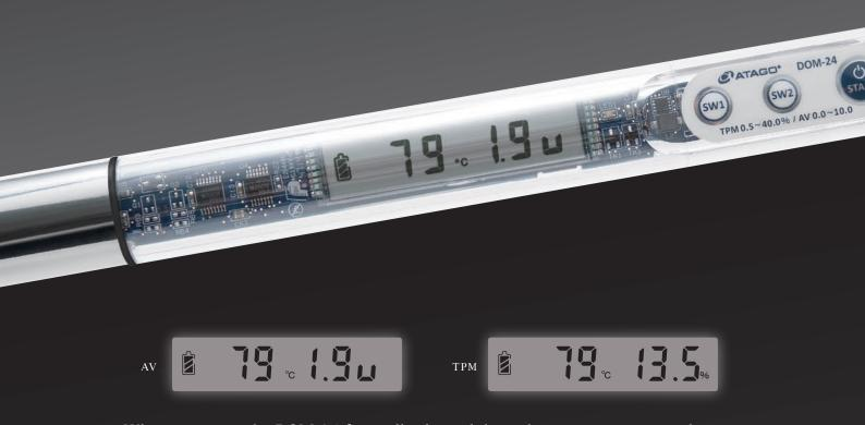
What separates the DOM-24 from all other oil degradation measurement devices is its ability to display Acid Value (AV).
