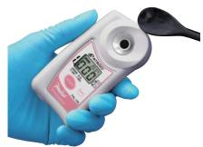
The PAL-10S is a digital hand-held compact refractometer that measures Urine Specific Gravity. To operate, simply place a drop of urine on the prism surface and press the START key. The Urine Specific Gravity value will be displayed on the LCD.
