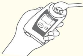
Place filter paper on the prism and place the soil-glycerin mixture on top.
